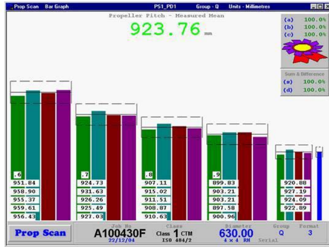
Figure 5 – Right handed propeller pitch measurements after tuning
