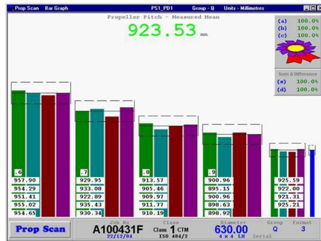
Figure 7 – Left handed propeller pitch measurements after tuning
