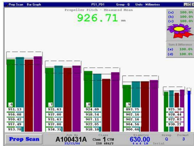
Figure 4 – Left handed propeller pitch measurements
